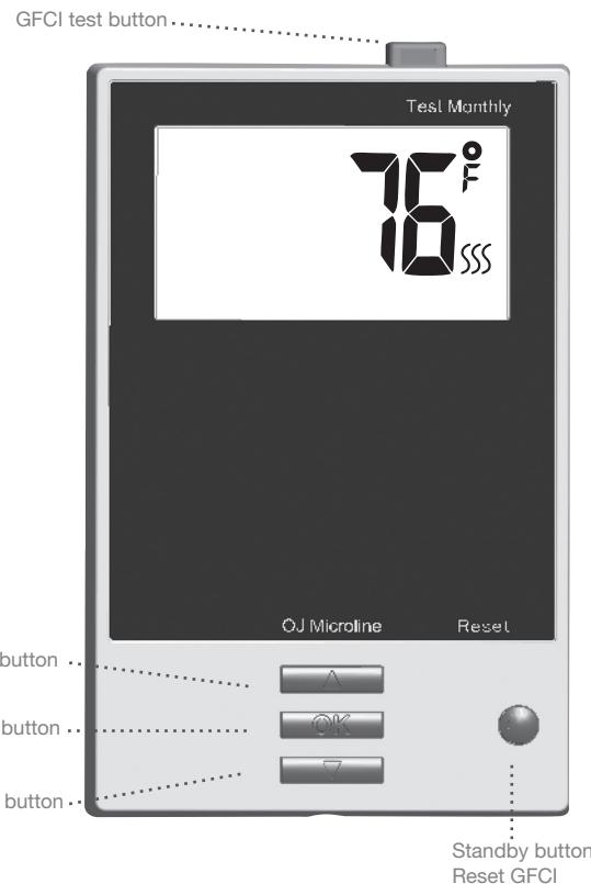
to the new setpoint. Then press the **TEST** button on the top of the thermostat. The test is successful if the red light in the **TEST** button lights up and **GROUND FAULT** is shown on the display. If this does not occur, check the installation/contact your electrical installer. Press the **Standby/Reset** button to reset the GFCI.
