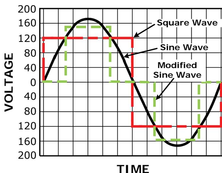
Figure 1-5, AC Waveforms
