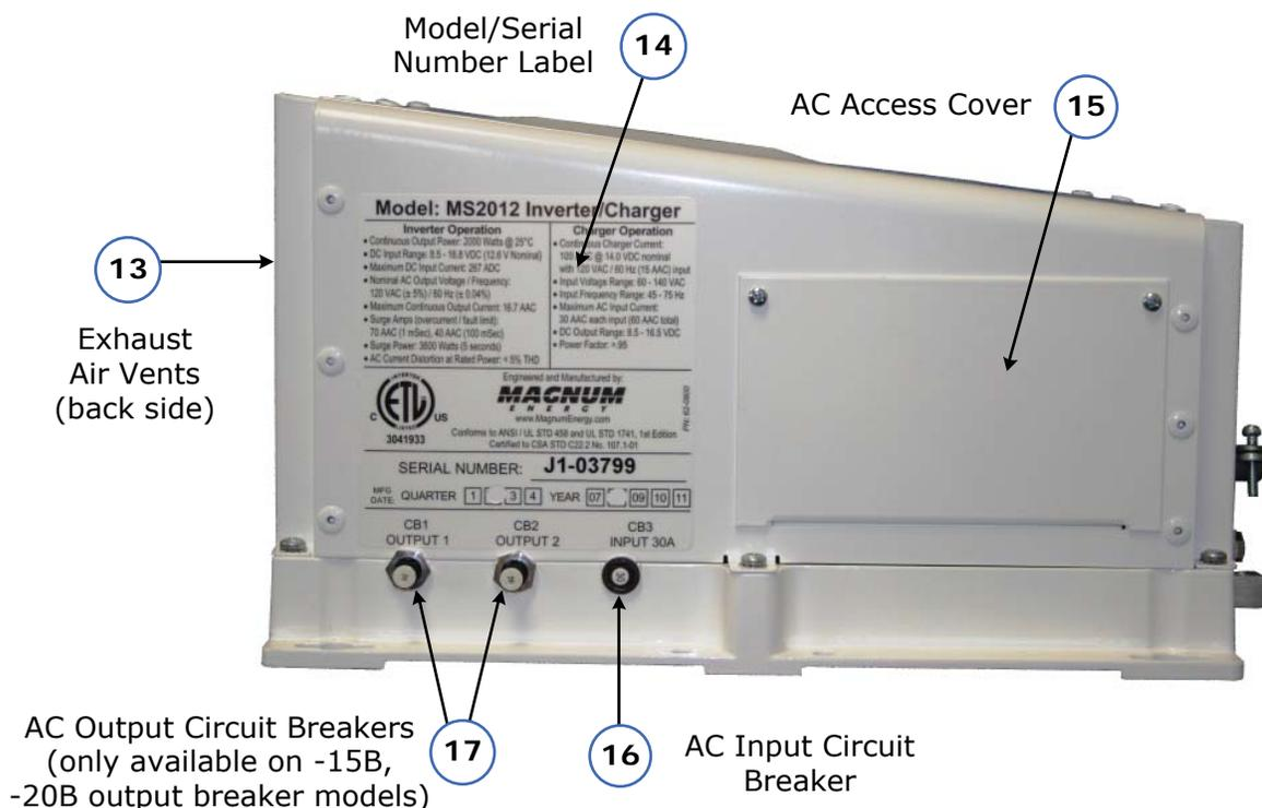
**Figure 1-3, Left Side Features (MS2012, MS2812, MS2024, MS4024)**
