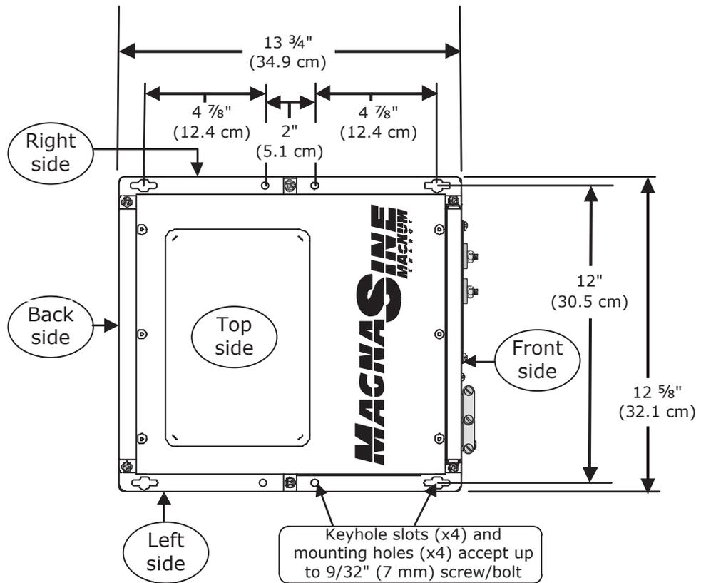
**Figure 2-3, MS Series Dimensions and Side Reference**
