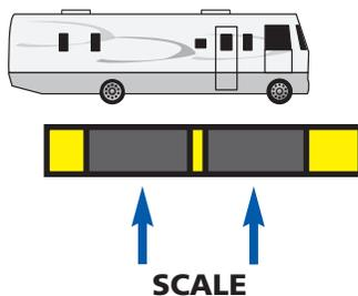
**3) Single Axle** – Weighs one axle at a time.
