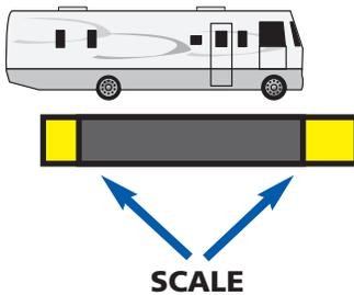
**2) Segmented Platform** – Platform scales with segmented sections can provide individual axle weights and total vehicle weights all at once when the vehicle is positioned properly.
