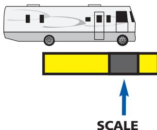
**Note:** Even though the weight of the total axle is within the axle rating, it may be overloaded on one side, which means an overloaded wheel position. That's why side-to-side weighing is required.
