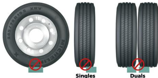
Incorrect One tire or only a portion of one tire is supporting the full load.
