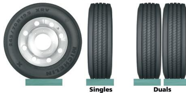
Correct Evenly supporting the full load.
