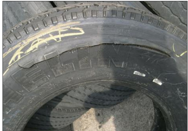
Fatigue Rupture or “Zipper”
