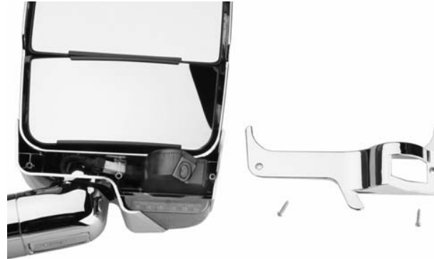
LEM with Cover plate removed
